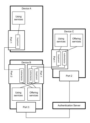
Figure 1 - Architecture of PBNAC system
