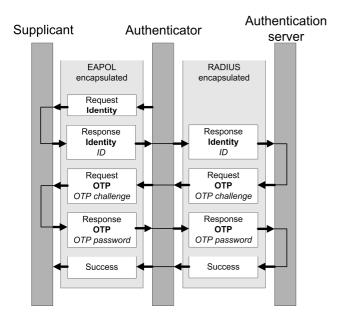
Figure 2 – Possible EAP communication
