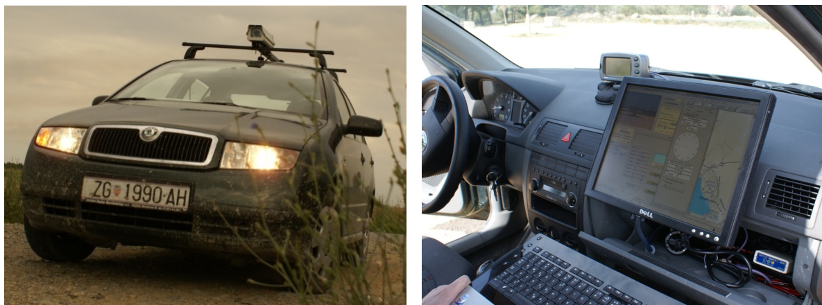
Figure 1. The vehicle used for acquisition of road videos. The videos are georeferenced using an on-board computer equipped with a geoinformation system.
