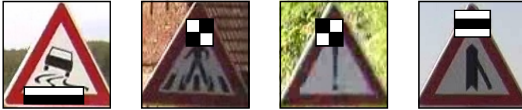
Figure 8. The first four features of cascade stage 1 superimposed on sign images.
