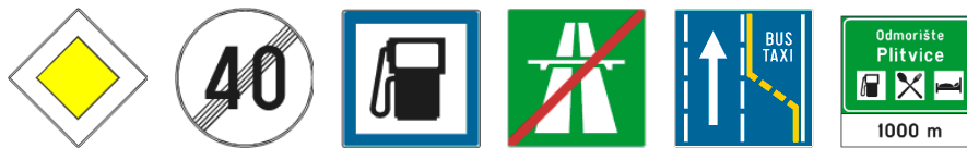
Figure 5. Examples of information traffic signs. Although their semantic use is the same – conveying information to the driver – their appearance can be very different.
