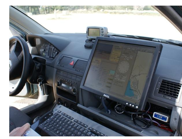
The road filming is done using a car equipped with a camera and a GPS receiver. The video is georeferenced in real time using an on-board computer.
