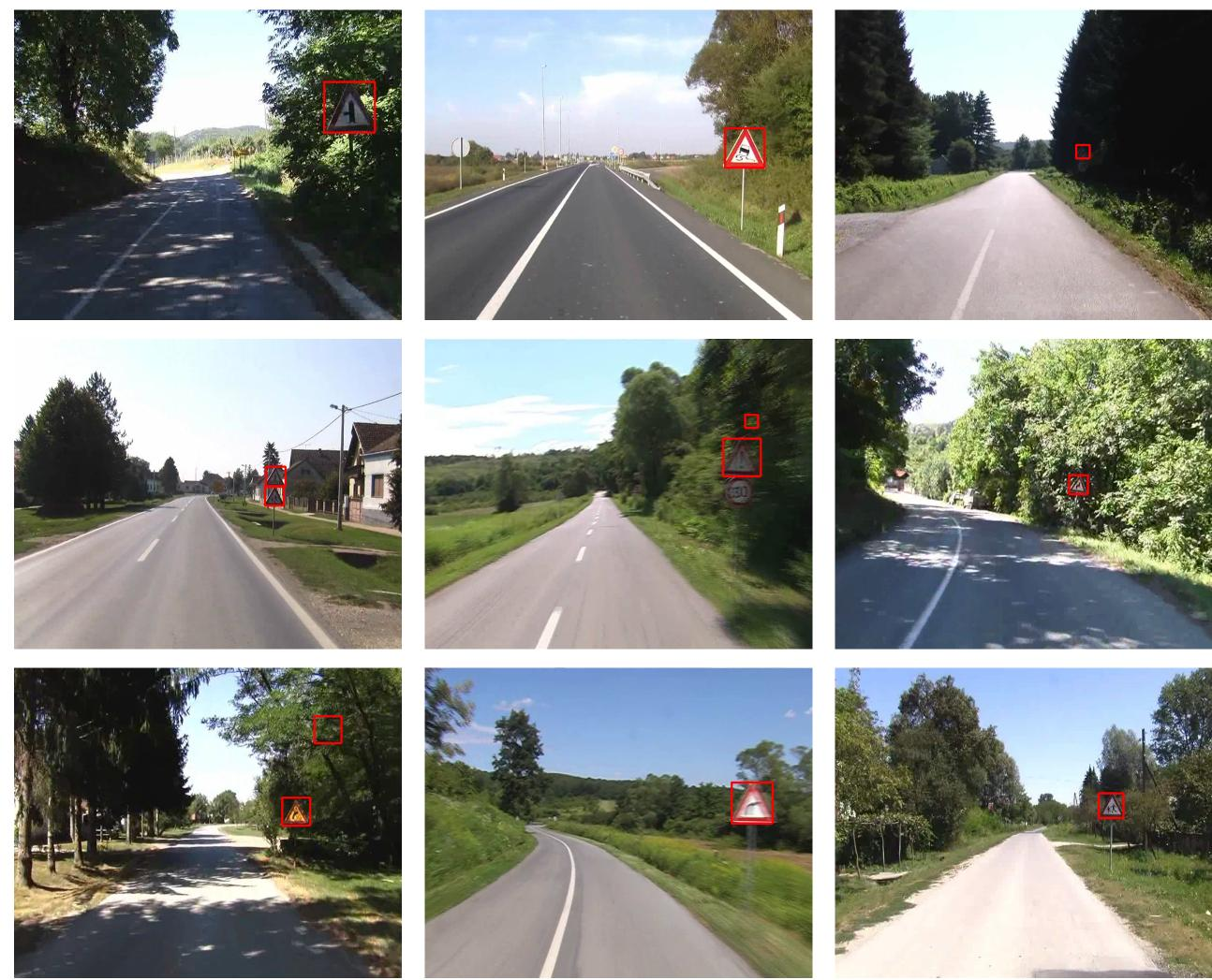
The detector is robust to the effects of motion blur, shadows and color inconsistency.
