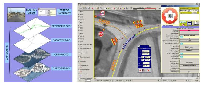
Fig. 2. Capabilities of the presented geoinformation system: some of the supported data layers (left), and a view of the traffic sign inventory layer shown above the ortophoto layer (right). Red circles in the right figure denote car positions during the mapping session.
