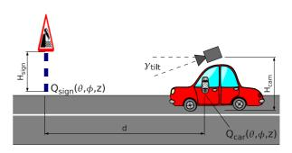
Fig. 1. Geometric relations between the camera, car, and the assessed road section ( $Q_{\rm sign}$  is recovered during mapping,  $Q_{\rm car}$  is measured).
