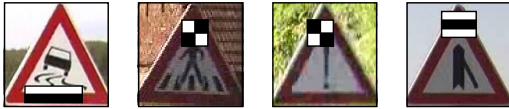
Fig. 6 The four features from the first stage of the cascade superimposed on typical images of traffic signs. The leftmost feature is sensitive to the bottom edge of a sign, while the other three detect the structure near the top of the sign.
