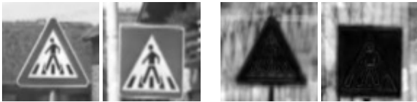
Fig. 19 Two similar signs with different shapes (left). The corresponding shape masks recovered from the motion sequences shown in Fig. 18 (right).
