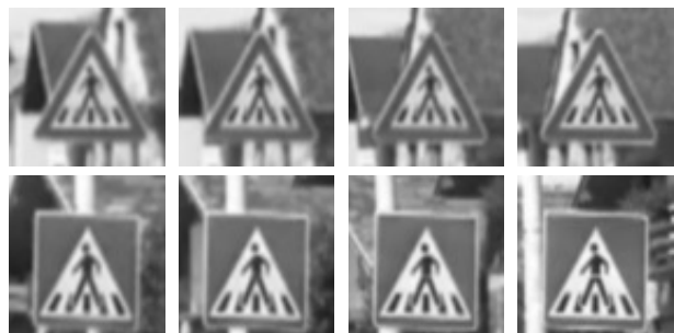
Fig. 18 Two traffic signs which are quite similar in grayscale appearance are easily distinguished in a motion sequence due to different occlusion boundaries. The shape difference is noticeable only when the two objects are observed in motion.
