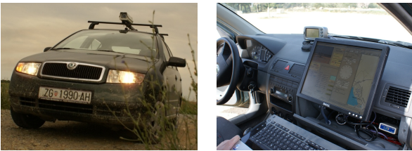
Fig. 4. The vehicle used for acquisition of road videos, equipped with a single camera, a GPS receiver and an odometer. The videos are geo-referenced using an on-board computer equipped with a geoinformation system.
