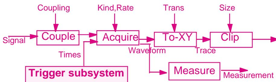
Figure 14: Oscilloscopes – A Modified Pipe and Filter Model
