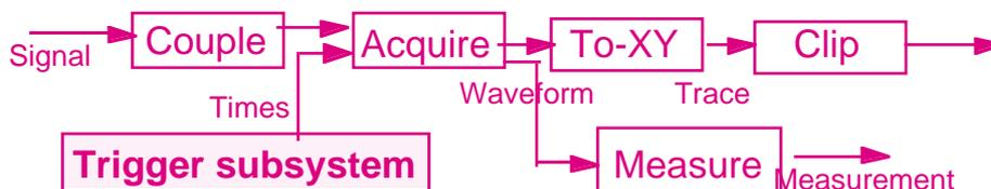
Figure 13: Oscilloscopes – A Pipe and Filter Model
