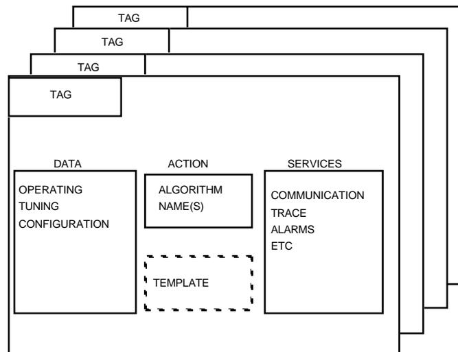
Figure 20: PROVOX – Object-oriented Elaboration
