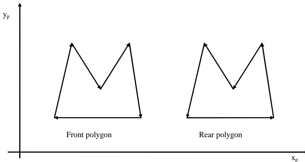
Figure 7.2. Determining rear polygons based on their orientation in the projection
