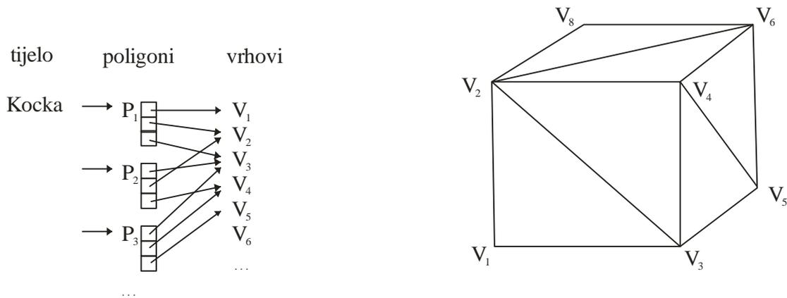
Figure 4.1. The body and the adherent data structures.
