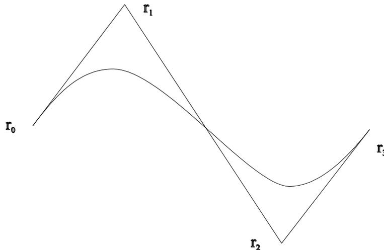
Figure 1. Example of a curve defined with four points.
