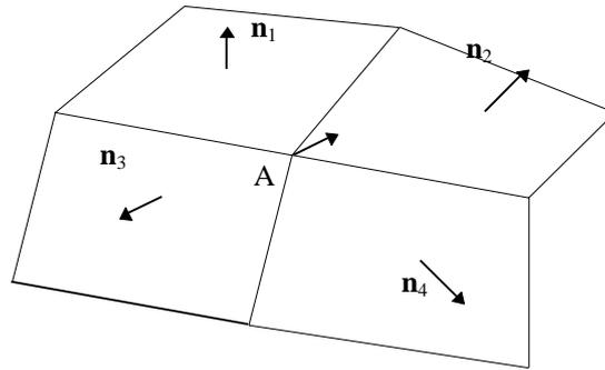
Figure 7.4 Determining the normal of vertex A.
