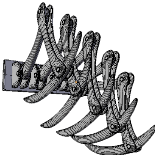
Figure 2.3: The five pick fingers used for plucking the strings. Each finger moves independently and can reach all five strings.
