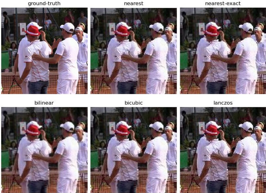
Figure 3.6: Comparison of different interpolation methods for upscaling from 128 \times 128 to 512 \times 512 . Particularly all methods struggle with fine sharp details like the net of the tennis court.
