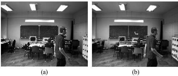
Figure 1. Successive frames with marked detected corner features and feature velocities obtained from matching process (the calculated dominant feature velocity is shown by the bold vector in (b)).
