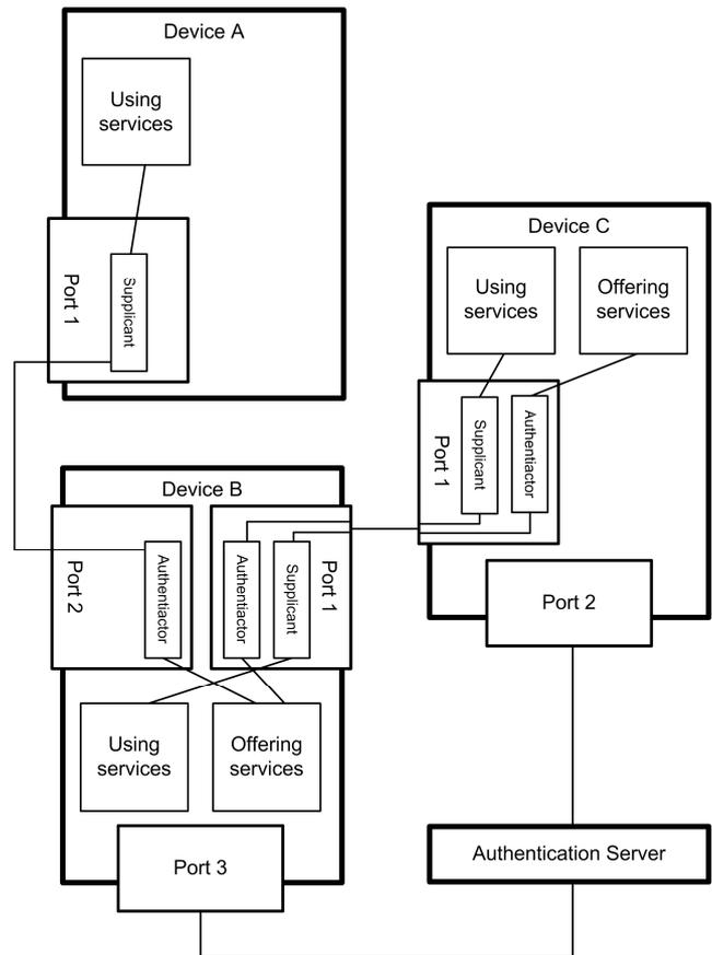
Figure 1 - Architecture of PBNAC system
