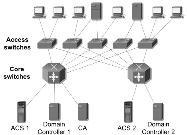
Figure 3 – Network of implemented PBNAC elements
