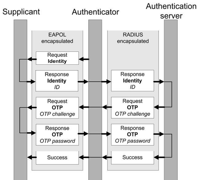
Figure 2 – Possible EAP communication
