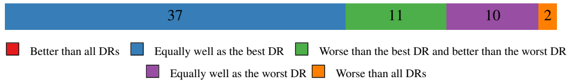
Figure 6.31: Performance of the best ensemble constructed by unweighted BoostGP and combined by using the vote combination method compared to the performance of individual DRs out of which it was constructed
