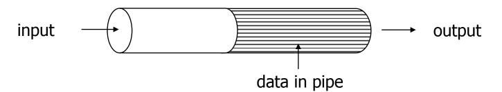
Data is sent to pipe through input side, and read from output side
