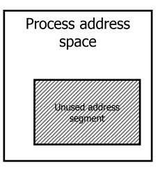
Unused memory space of a process can be reserved as address segment for shared memory object using system functions.
