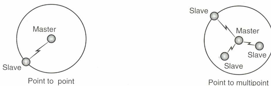
Slika 6. Point to point i point to multipoint piconet .
