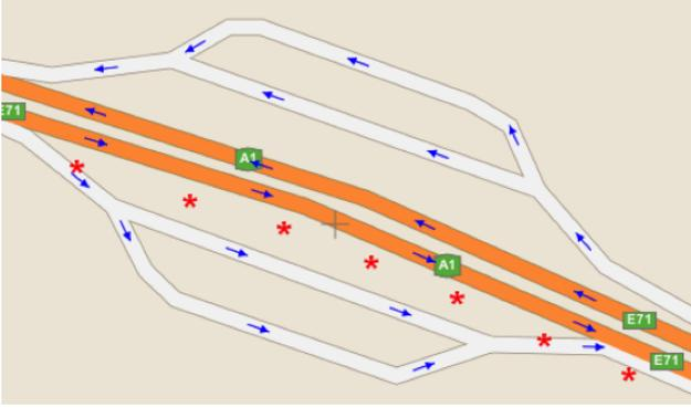
Figure 3: Ambiguous route reconstruction due to poor GPS precision. GPS readings are marked with red asterisks. It is equally plausible that the vehicle travelled the highway (in orange) and the local road (in white).
