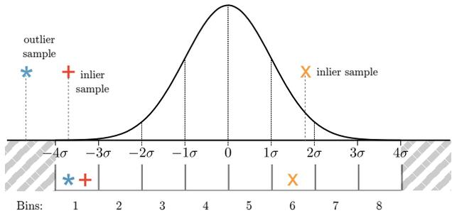
Figure 5: The encoding scheme for  $N = 3$  bits and the interval width of  $w = 4\sigma$ . The closed interval  $[-4\sigma, 4\sigma]$  is split into  $2^3 = 8$  equally wide bins. Value mapping is illustrated for three samples (orange, red and blue). Note that the values outside the interval (the blue asterisk) are mapped to the nearest bin.
