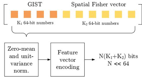
Figure 4: Our method: after obtaining shortened GIST and spatial Fisher vectors descriptors (of lengths  $K_1$  and  $K_2$ , respectively), their concatenation is normalized to zero mean, unit variance. Each component of the result is then encoded using only  $N$  bits, so the total size of the output is  $N(K_1 + K_2)$  bits.
