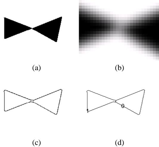
Figure 1: A synthetic test image (a), the enlarged central portion of the image smoothed with  $\sigma = 2$  (b), the edge map provided by the Canny edge detector (c), and the extracted canonical set of 2 closed contours (d) labeled with “0” and “1”.
