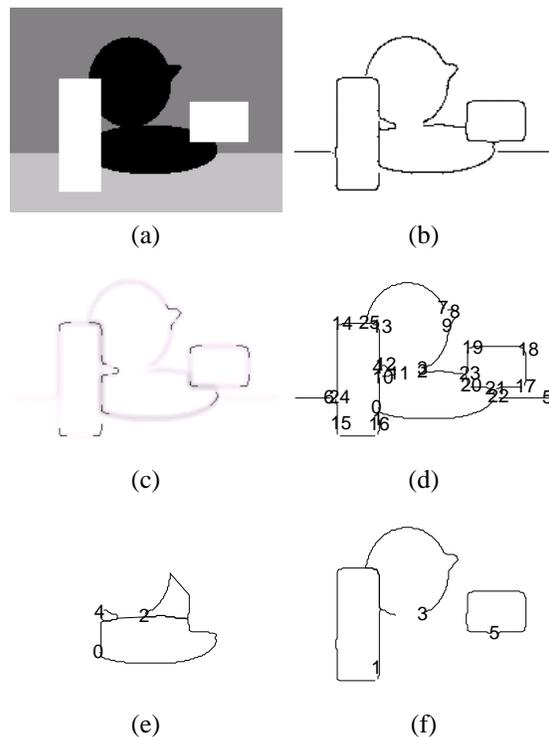
Figure 3: A complex synthetic test image (a), its edge map (b), the points of high curvature at which the chains are broken superimposed to the gradient image used by the edge detector (c), the final set of 30 edge chains (d), and finally, the obtained canonical set of 6 closed contours (e) and (f). In both contours #0 and #3, one large interruption is tolerated.
