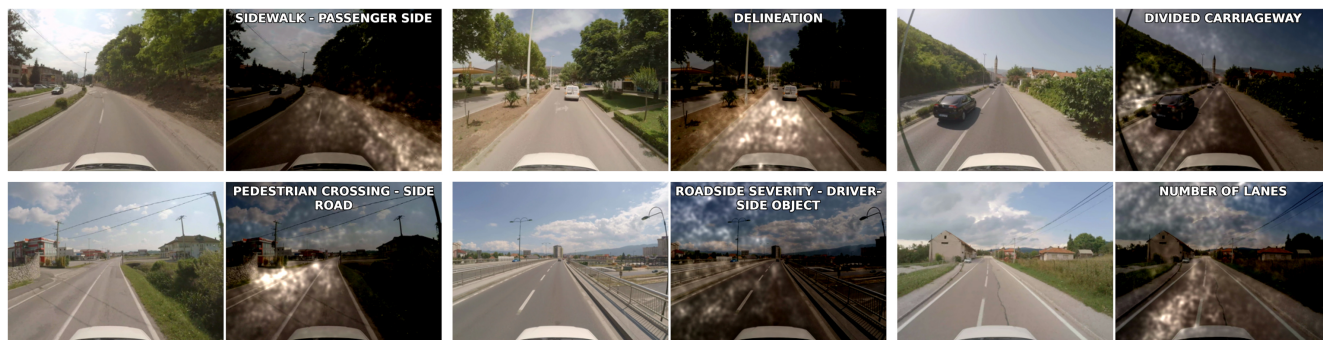
Fig. 2. Each image pair highlights regions which are responsible for the model decision. As shown in the images, the chosen attributes are, respectively: Sidewalk - passenger-side, Delineation, Divided carriageway (top), and Pedestrian crossing - side road, Roadside severity - driver-side object, and Number of lanes (bottom).
