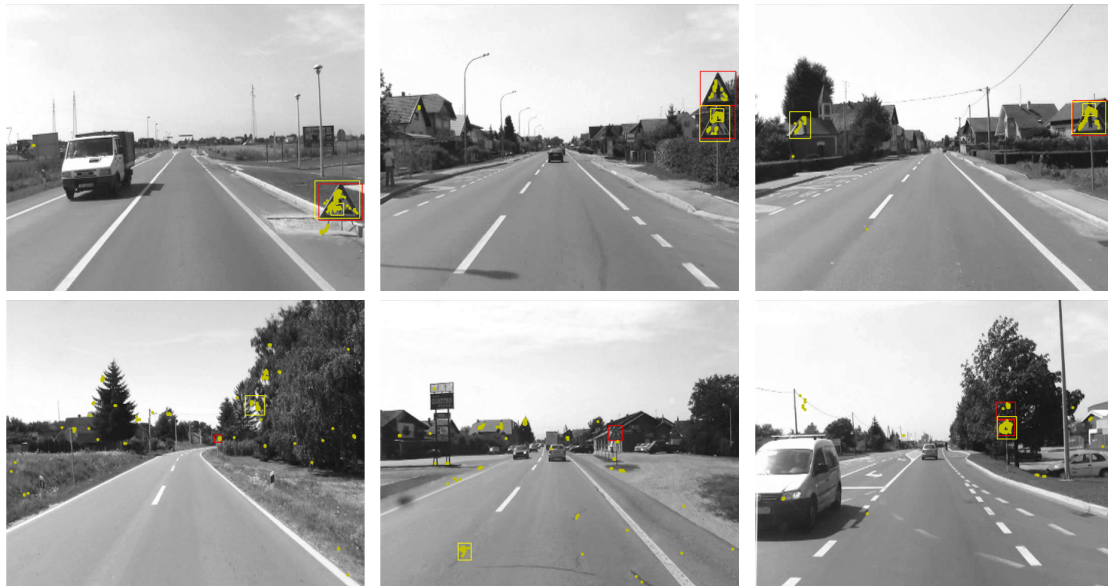
Figure 5: Detections counted as false alarms (top row), and missed detections (bottom row). The main causes of false alarms are insufficient overlap with the groundtruth location and background structures similar to warning signs ( e.g. roofs). Most missed signs are either small or contain out-of-plane rotations which are seldom encountered in the train split.
