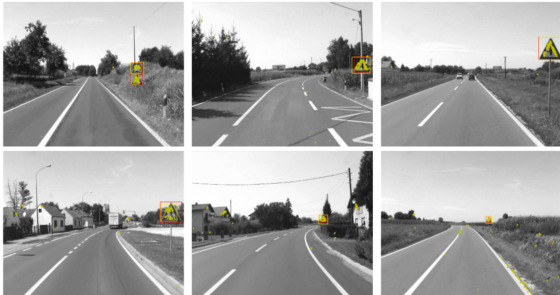
Figure 4: Successful operation: the method is able to detect multiple objects (cf. top-left) and to handle the complex background and small objects. Yellow dots indicate top ranked patches (rank < T ), yellow rectangles show the detected bounding boxes, while red rectangles indicate the groundtruth locations (which are used exclusively for evaluation).
