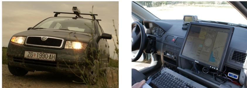
The road filming is done using a car equipped with a camera and a GPS receiver. The video is georeferenced in real time using an on-board computer.
