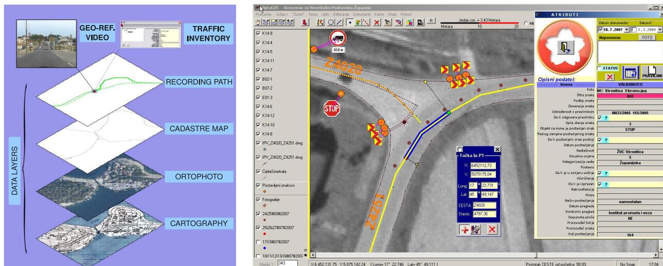
Fig. 2. Capabilities of the presented geoinformation system: some of the supported data layers (left), and a view of the traffic sign inventory layer shown above the ortophoto layer (right). Red circles in the right figure denote car positions during the mapping session.
