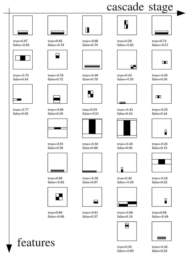
Fig. 9. The first five stages of the cascade obtained with basic set of features and symmetry on. Columns correspond to individual stages of the cascade. Numbers under each feature indicate influence of the feature to the compound result of the stage classifier, in cases of the positive (*true*) and negative (*false*) outcome. A candidate region is detected as triangular traffic sign if it passes all stage classifiers.
