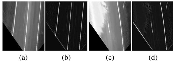
Fig. 6. Two inverse-perspective images (a,c), and the corresponding steerable filter responses (b,d).
