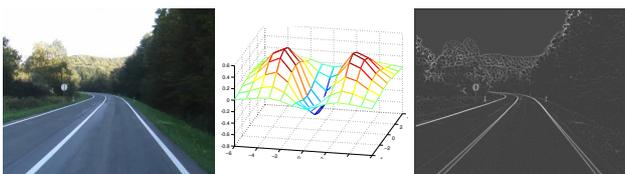
Fig. 5. Original image (left), steerable filter  $G_{xx}$  (middle), and the corresponding response (right). The scale of the employed filter does not suit the lane width in the bottom of the image, resulting in a “hollow” response.
