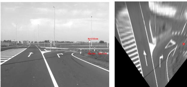
Fig. 4. Source image acquired from the driver's perspective (left) and the corresponding inverse-perspective image (right).
