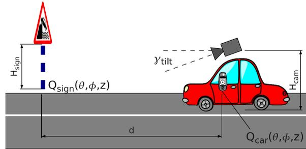
Fig. 1. Geometric relations between the camera, car, and the assessed road section ( $Q_{\text{sign}}$  is recovered during mapping,  $Q_{\text{car}}$  is measured).
