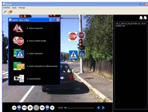
Fig. 7. A sign instance is annotated by (i) enclosing it in a bounding box, and (ii) selecting the sign type.
