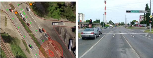
Fig. 5. The schematic view of the traffic inventory (left), and the corresponding georeferenced video frame (right) as presented by OptaGIS.
