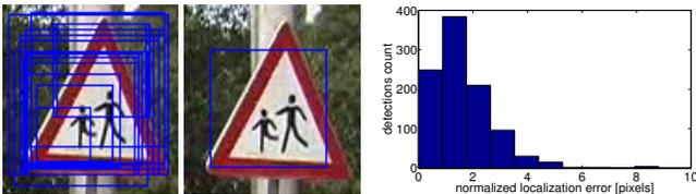
Fig. 9. The response of the grouping algorithm often deviates from the true location of the sign (left). The distribution of the relative deviations on the set T2010 normalized for the sign dimensions of  $24 \times 24$  is shown on the right.
