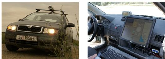
Fig. 1. The vehicle used for acquisition of road videos, equipped with a single camera, a GPS receiver and an odometer. The videos are georeferenced using an on-board computer equipped with a geoinformation system.
