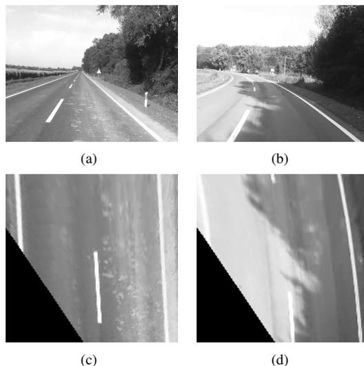
Fig. 2. Images captured from a moving vehicle (a,b) and the corresponding inverse perspective mappings (c,d). Different configurations of the road are shown: a straight road (a) is transformed into the orthogonal image (c), a slightly curved road (b) is transformed into the orthogonal image (d).
