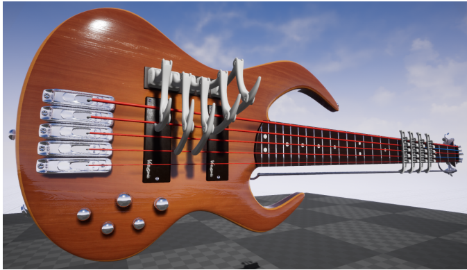
Fig. 6. The bass model with picking and fretting mechanisms imported into Unreal Engine. The strings are colored red and blue in order to help visualize the material change when a string is bent to a fret using a shape key.
