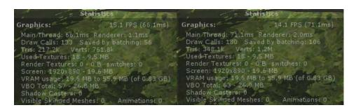
Figure 2.3: Left - forest scene using OC, Right - same forest scene without OC A small part of the forest is hidden by a hill, OC knows this so it doesn't send those trees to render which we can see by the lowered draw call count, triangle count and render time
