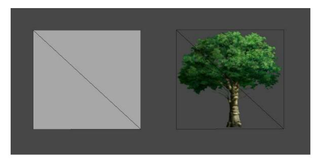
Figure 1.2: Left – a simple billboard consisting of two triangles, Right – same billboard but with a transparent texture applied
