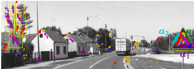
Fig. 1. The appearance model identifies distinctive patches (enclosed in yellow rectangles) assigned to selected visual words (shown in colors). The spatial model learns consistent spatial configurations between pairs of selected visual words, e.g. between a_1 (purple) and a_2 (cyan), a_1 (purple) and a_3 (green) and so on.
