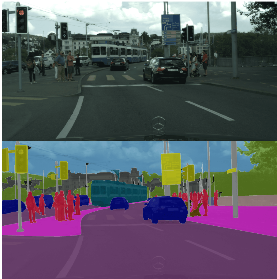
Figure 2.10: Semantic segmentation example. The top image is the input image, the bottom image is the ground truth segmentation. Each colour represents a separate class. A segmentation model doesn't directly produce an output shown on the bottom. Instead the problem is often modeled as a pixel-wise classification problem, where the output is of the shape (C \times W \times H) , with C being the number of classes. The images were taken from the Cityscapes dataset [1].
