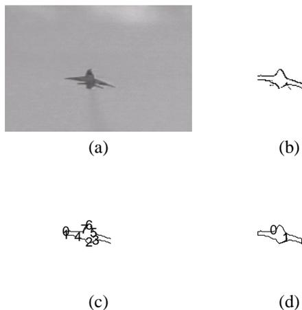
Figure 4: A simple real image (a), its edge map (b), the final set of 8 edge chains (c), and the obtained canonical set of 2 closed contours (d). In both contours, one apex is tolerated.
