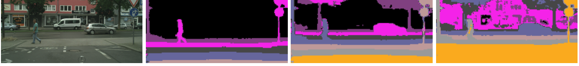
Figure 3.2: Visualization of the scale selection switches. From left to right: original image, switches for the three reference metric scales of 1m, 4m and 7m.
