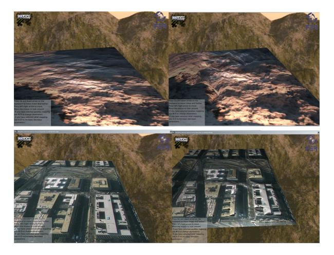
Figure 5. Texture mapping (left) and relief mapping (right).
